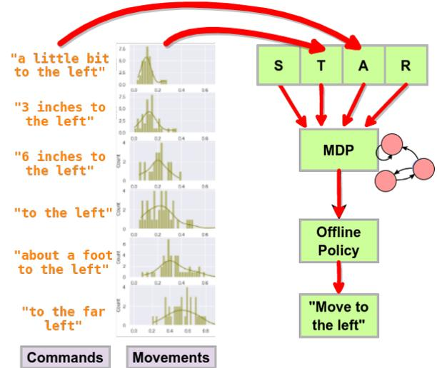
Fig. 4: From left to right: A sample of discrete commands. The movement (in meters) each command caused. We learned a model of human hand movement from demonstrations that gave us the transition probabilities  $T$ .  $S$  defines the state space,  $A$  defines the discrete set of verbal actions, and  $R$  is the reward function. A policy is learned offline that can be used across reaching tasks.
