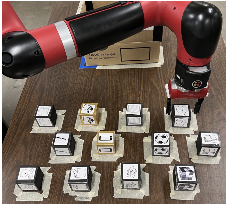
Fig. 3: The robot picking up an item from its workspace to be placed into the box for the order-fulfillment task. The cubes with gold backgrounds (e.g., laptop in the top row) are high value items.
